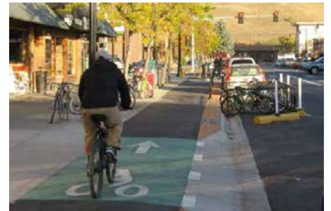
RAISED TRAIL WITH PAINTED DRIVEWAY CROSSINGS SOURCE: CITY OF MISSOULA
